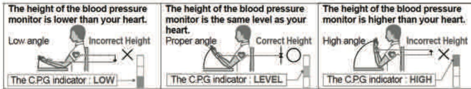
The position of the device is checked both before and after measurement.
